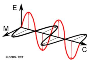
All electromagnetic radiation has fundamental properties and behaves in predictable ways according to the basics of wave theory. **Electromagnetic radiation** consists of an electrical field(E) which varies in magnitude in a direction perpendicular to the direction in which the radiation is traveling, and a magnetic field (M) oriented at right angles to the electrical field. Both these fields travel at the speed of light (c).
